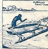
OUTRIGGER CANOES. Outrigger canoes are to be found all about the islands of the Pacific Ocean. The sim- plest form is that illustrated from Australia—a hollowed out tree trunk with outrigger attached to give balance.
